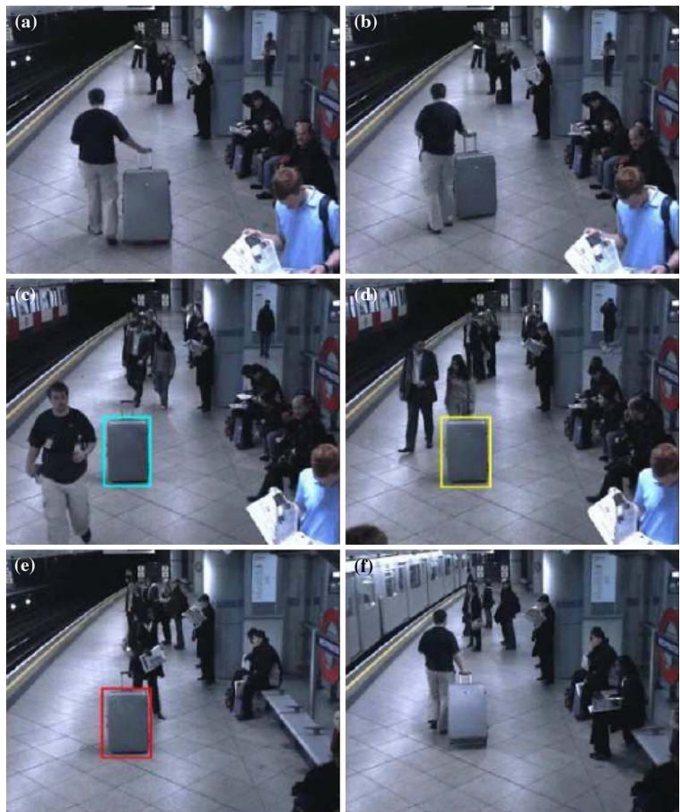
Fig. 6 Results of processing sequence Test4_i-LIDS. The unattended baggage is first identified in c , which initiates reverse traversal up to b where the baggage is not found at the detected location. Tracking the moved baggage backward in time to a where a sufficient number of the owner's appearance patch is collected. Returning to the point when unattended baggage is discovered, d shows the complete departure of the owner, which enables the timer. 60 s later, the alarm is triggered ( e ), and is eventually set off ( f ) by the owner's return
