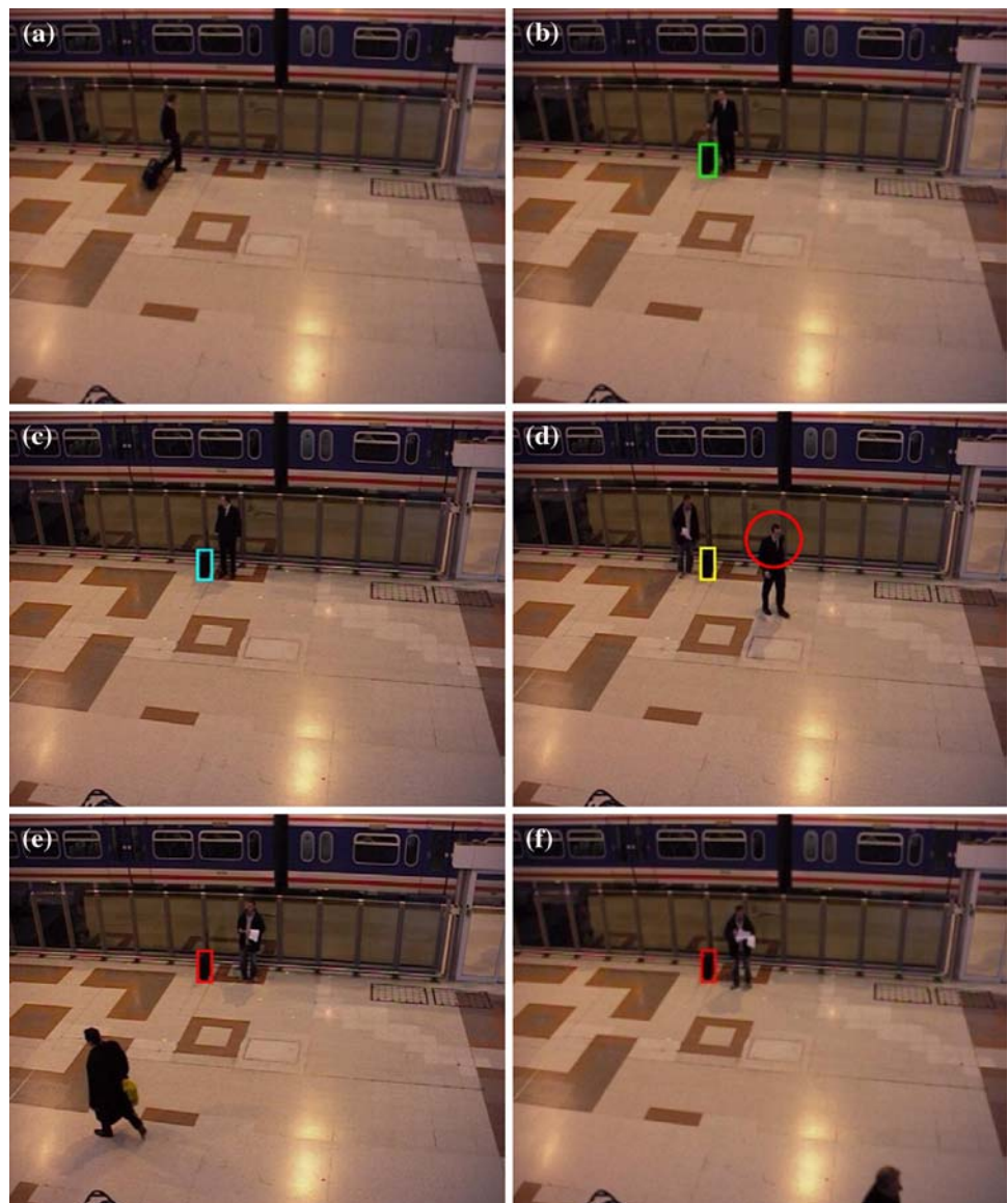
Fig. 7 Snapshots of the process of sequence S4C3_PETS06. In c the baggage is not in physical contact with the owner, and is locked on by the unattended object detector. The system traverses backward in time to search for the initial presence of the baggage. b to a , image patches are collected from the foreground area around the detected baggage. In d , the departure of the owner (marked by red circle ) from the baggage neighborhood (defined in PETS 2006) starts the timer. Since the owner never comes back to the scene after his leaving, the alarm continues from e to f (the last frame) (colour in online)
